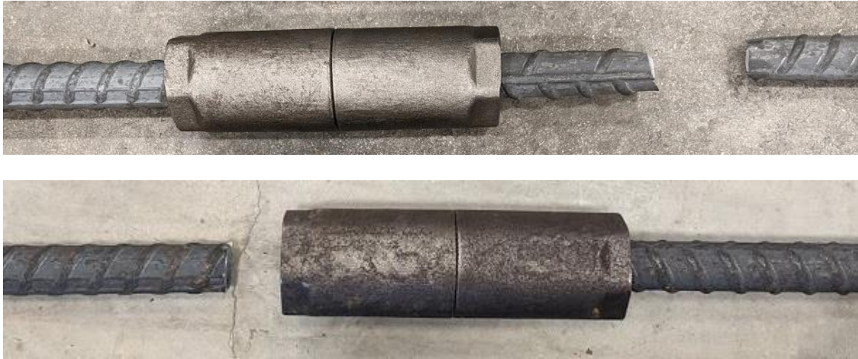
Figure 3. Representative fractured spliced bar test specimens. Top: Bar fracture away from the coupler. Bottom: Bar fracture at indentation in bar created by the wedges internal to the coupler.
